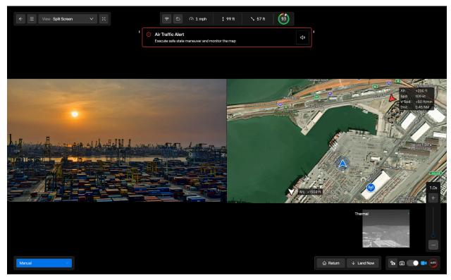
Example of Air Traffic Alert in Skydio Flight Deck Drone as First Responder (DFR) software.
