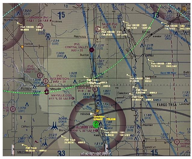
Airspace awareness displays with radar data can be difficult for pilots to interpret, requiring additional training and experience. In this example, ADS-B data is shown with Primary Surveillance Radar (PSR). PSR targets have unknown altitudes with 2D radars.
